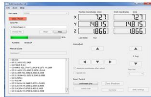
Fig 6.3 CNC control software window
