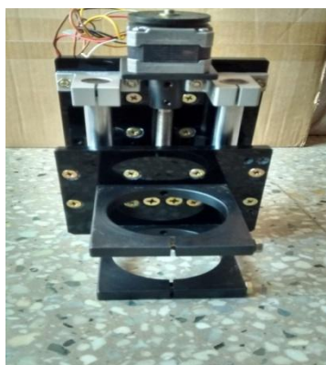
Fig 7.1 Z-axis assembly machine
